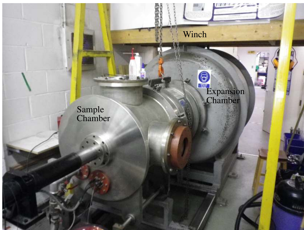
Figure 3.3 The sample and expansion chambers of the gas gun. A winch is used to raise a removable section of the chamber for loading the sample. At the bottom end of the sample chamber, the optical fibre for the PDV, and wires for other diagnostics, can be seen.
