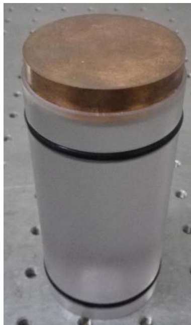
Figure 3.4 The projectile used in the gas gun has two rubber O-rings: the top one separates the barrel vacuum from the pressurised gas reservoirs and the bottom one separates the reservoirs from the rear holding vacuum.
